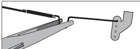
**For best performance with AS3X, it is important that excessive trim is not used.** If the aircraft requires excessive transmitter trim (4 or more clicks of trim per channel), return the transmitter trim to zero and adjust the linkages mechanically so that the control surfaces are in the flight trimmed position.
