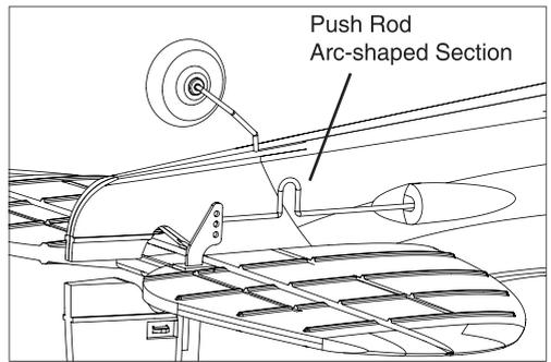
If the elevator is angled off to the upper or lower position, adjust the push rod by its arc-shaped section slightly, making sure the elevator is properly centered.
