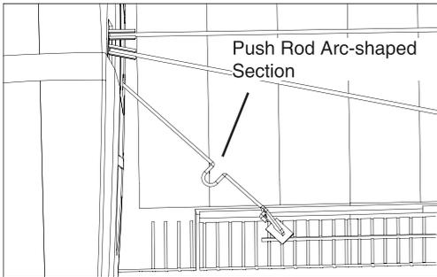
If the aileron is angled off to the upper or lower position, adjust the push rod by its arc-shaped section slightly, making sure the aileron is properly centered.
