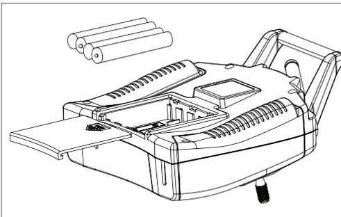
1. Install 4 AA batteries(not included) in the transmitter.
