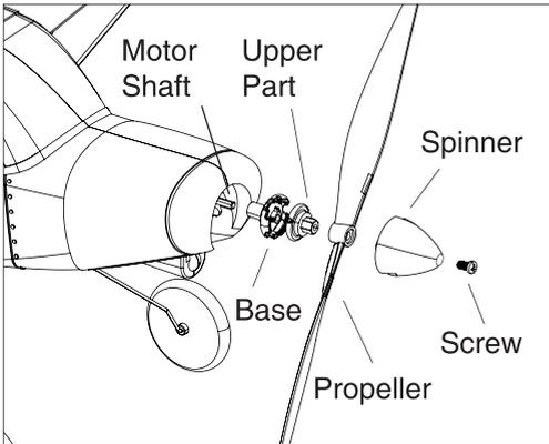
Follow below steps to replace broken propeller and shaft adaptor. You will need help of a Philips screw driver and pliers(not included).
