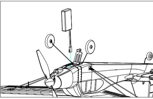
3. Connect the battery to the receiver, then stick the battery into the cabin, making sure the battery is well secured.
