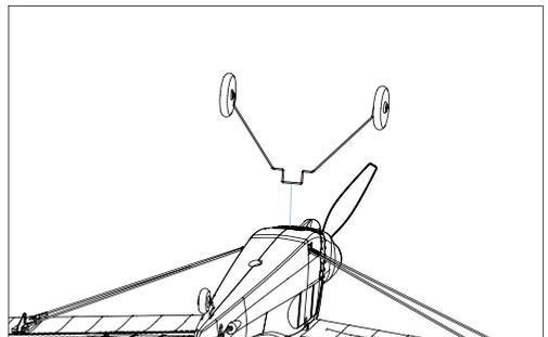
2. Plug the landing gear into the fuselage as shown above.
