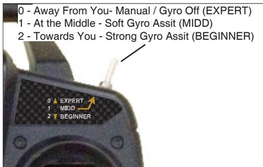
The Sport Cub S2 comes with pre-installed Gyro to help control flying easily.
