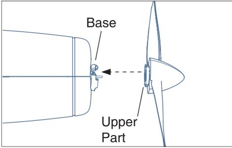
The propeller saver keeps the propeller from damage, and prevent the electronic components from over current. When the airplane hits any obstacle, the propeller will loose from the base. To install the propeller back to the base, insert the upper part centerly through the motor shaft, and hearing a "click" sound to ensure it is secured.
