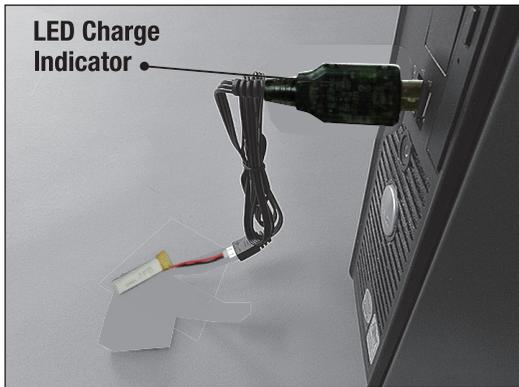
4. The charging process takes about 3.5 hours. For safety reasons, never charge the battery for longer than 4 hours. While charging, the red LED indicator will be flashing. When the charging is finished, the red LED will be off.
