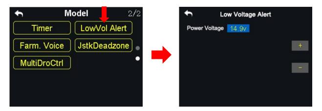
When the user's aircraft power voltage is lower than the safe level, the DK32S transmitter will vibrate and send voice alert.
