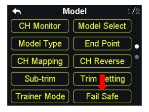
Before linking the DK32S transmitter to the sky station, do not forget to do fail-safe settings and turn on the function. Thus if the transmitter lost link with the sky station, the fail-safe function will run automatically and immediately to protect the aircraft from a crash.
