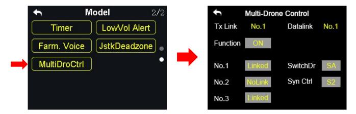
Through one DK32S transmitter users can control up to three drones at the same time.
