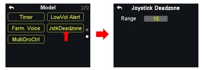
By setting a certain dead zone range, the DK32S transmitter helps user filter out channel values which are input by touching the joysticks unintentionally.
