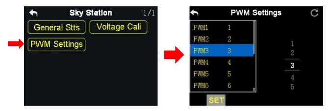
In the DK32S transmitter and the PWM mode, users can redefine the output channel of the sky station (channel 1-9 in default), so that if the channel 9 is already working in SBUS or PPM mode, the PWM ports 1 to 8 can still output to the channels 1 to 16 of the transmitter.
