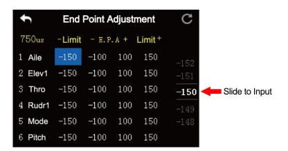
3. Select a channel and its output value, press the "+" or "-" button on transmitter to adjust value or limit  $(-150 \sim 150)$ .
