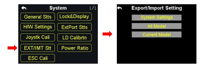
Through the export setting function users can export the data of system settings and model settings to the SD card so as to share the data to another DK32S transmitter.
