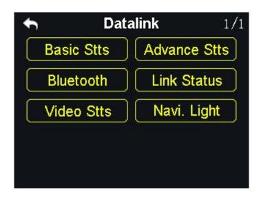
Basic Stts (Basic Settings): Set basic functions of the datalink module.
