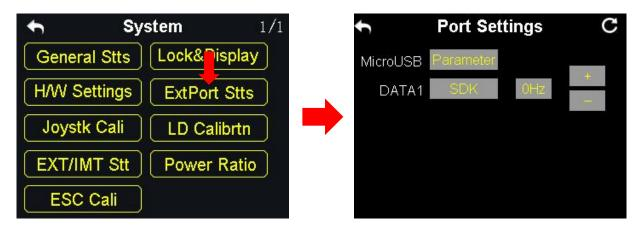
The extending ports function help users extend transmitter function to external hardware devices and SDK. Currently the DK32S transmitter supports a Micro-USB port, a USB port and a 4-Pin Groove Port (DATA1).
