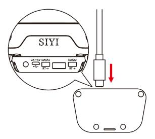
Please us original OTG Micro-USB cable coming in DK32S packing list to plug into the Micro-USB port on transmitter and the USB charger.
