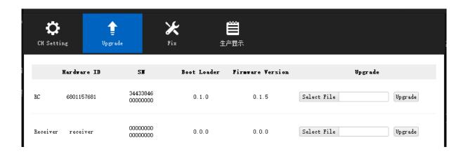
When the ground unit RF firmware and the air unit RF firmware are different in initial numbers, they can still bind and work normally as long as their firmware version actually match.
