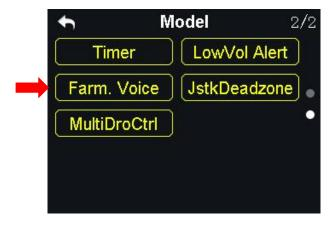
The Farming Voice is a professional function is for farming drones. The function is supported by up to 6 switches with 16 positions. They are SA, SB, SC, SD, S2 and S3.
