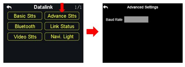
If your flight controller type was not in the list, you can set a baud rate to match your flight controller.
