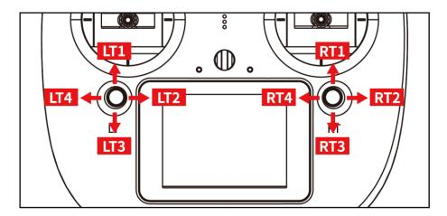
There are 2 Sub-Trim buttons on DK32S transmitter, which support continuous trimming to all 4 channels.
