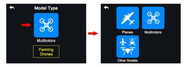
3. Tap on a model type according to your requirement, then "Apply" to finish.
