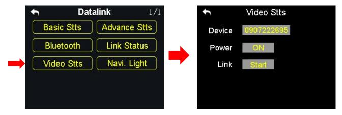
Users can check the serial number of the video transmission module and power on/off the function.
