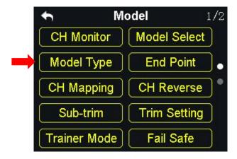
In the DK32S transmitter there are several default model types, Fixed-wings / Gliders, Multi-rotors (racing drones, agricultural drones) and the others (helicopters), each model type with its default settings done in advance. Users can choose a model type according to their requirement and customize the settings.
