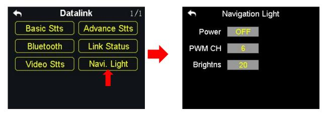
Users can power on/off the navigation light on the drone.
