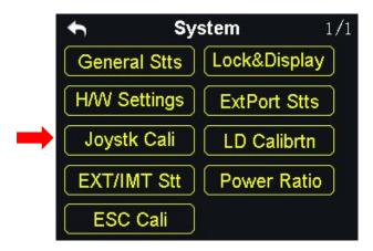
The Joystick calibrating function help users calibrate the joysticks' middle position.
