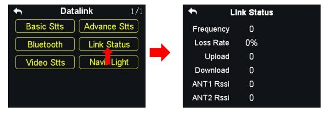
The link status function helps users check the detail signal and link status of the DK32S transmitter in real-time.
