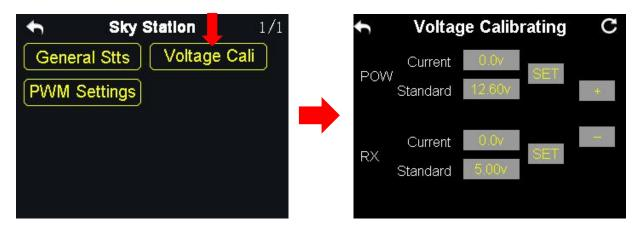
Before using the sky station, it is necessary to calibrate the telemetry voltage of both the sky station and the aircraft.
