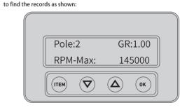
ratio is around 9.23. And Formula 100% throttle speed of the main rotor=MAX RPM ÷ (motor poles ÷ 2) ÷ gear ratio
