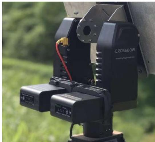
2. The antenna has to be mounted on the Crossbow AAT with the use of a special bracket. In order to prevent tampering with the normal operation of the compass built into the Crossbow AAT it is recommended to avoid using antennas made with ferromagnetic materials. Wherever possible, use non-magnetic stainless steel bolts, aluminum and other non-magnetic materials.
