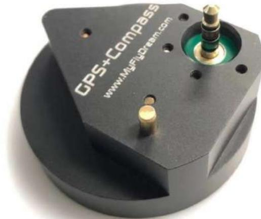
The Crossbow will recognize the GPS+Compass module once it's plugged. The screen will display something like GPS:12/L14 to show the number of satellites locked by remote GPS/ local GPS. With this module, The tracker will start to track when it locks enough satellites without setting home operation.
